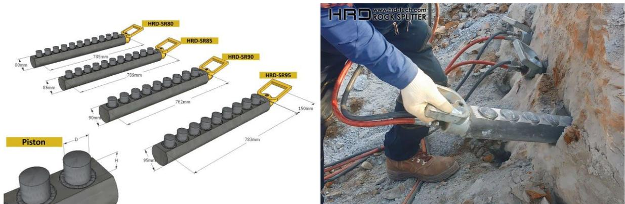
Figure 5: Splitting rods and an application example (Hwacheon HRD-TECH, 2017).
