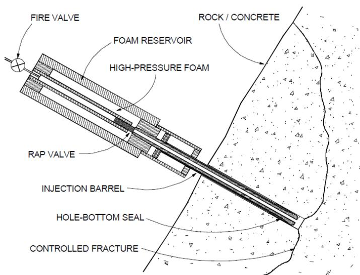
Figure 2: Controlled foam injection for rock fracturing, Chapman (1999).
