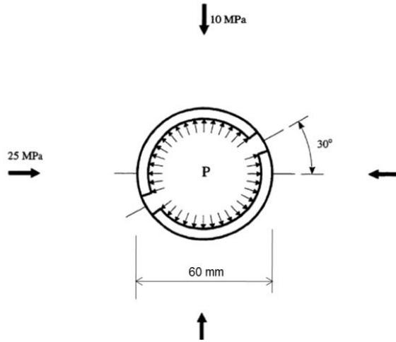
Figure 16: Configuration and loading condition of the numerical model (Backer, 2000)
