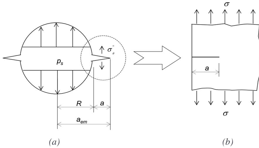
Figure 15: A crack on in a borehole wall (a) can be simplified to an edge crack in a semi-infinite body (b)
