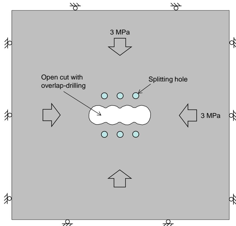
Figure 28: Configuration of open cut and numerical model for simulation
