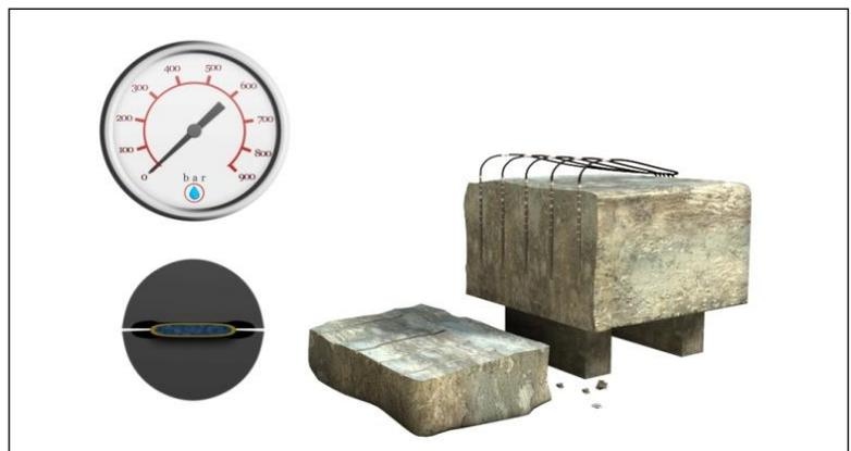
Figure 8: Working procedures for the hydraulic rock splitter
