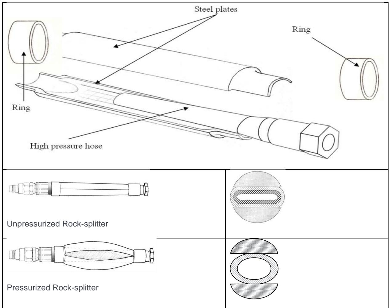
Figure 7: Hydraulic rock splitter used in this project
