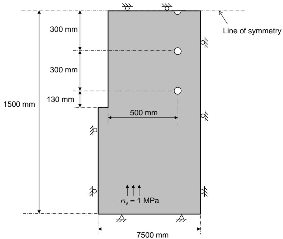
Figure 23: Model configuration for simulating hydraulic splitting with a free surface
