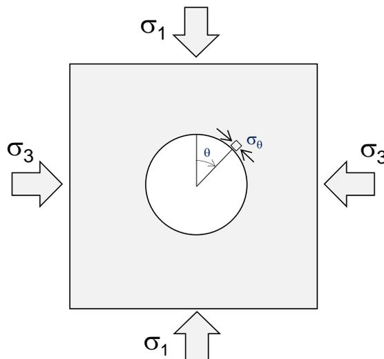
Figure 10: Stress situation surrounding a circular hole in a stressed elastic body
