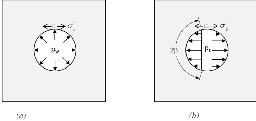
Figure 11: Tangential stress caused by internal pressures inside a circular borehole
