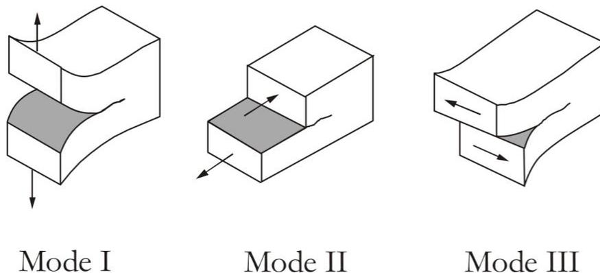
Figure 14: Basic modes of fracturing in rock (from Hudson & Harrison, 1997)
