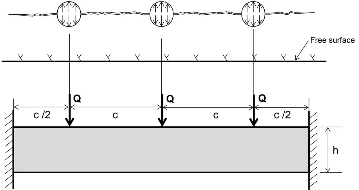
Figure 19: Model for estimating required load to break down the rock beam
