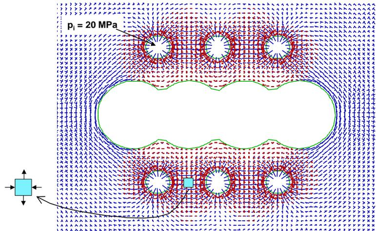
Figure 29: Stress distribution at 20 MPa pressure in the splitting holes (tensile stress in red colour)
