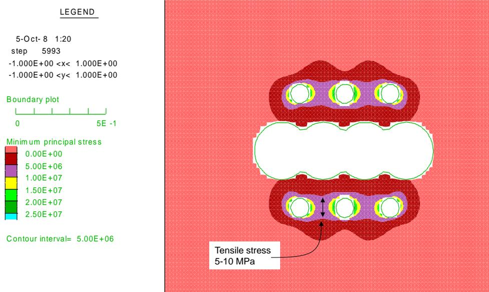
Figure 31: The minor principal stress  $\sigma_3$  at 20 MPa pressure in the splitting holes
