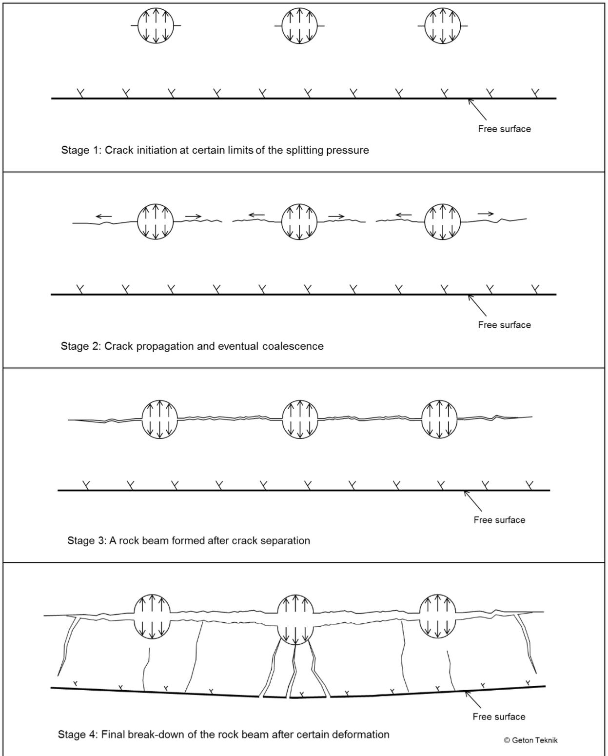
Figure 9: Process of hydraulic splitting with a free rock surface
