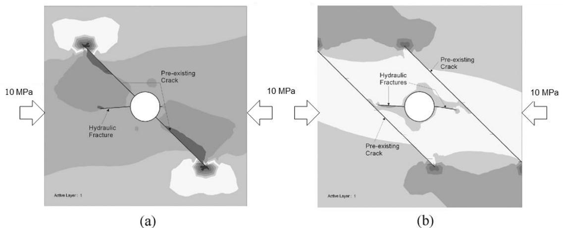
Figure 18: Numerical model for crack propagation with existing cracks
