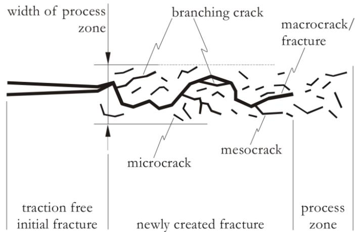
Figure 13: Fracture process zone (FPZ) consisting of micro- and mesocracks. (modified from Liu et al., 2000)
