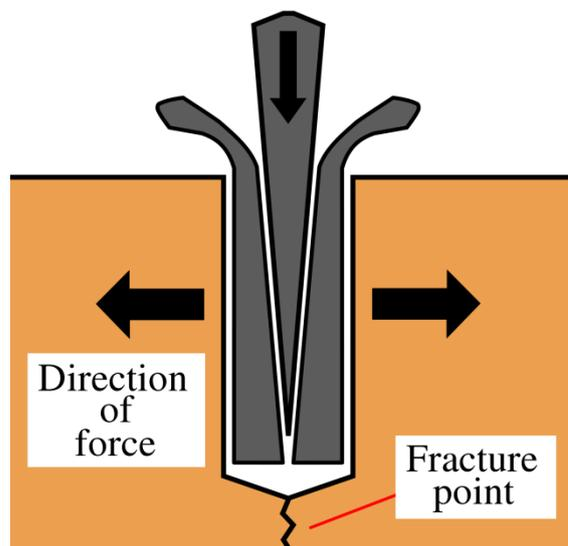
Figure 4: Principal of mechanical wedges.
