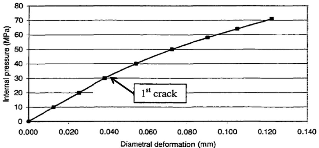
Figure 17: Calculated curve for applied internal pressure and radial deformation (Backer, 2000)
