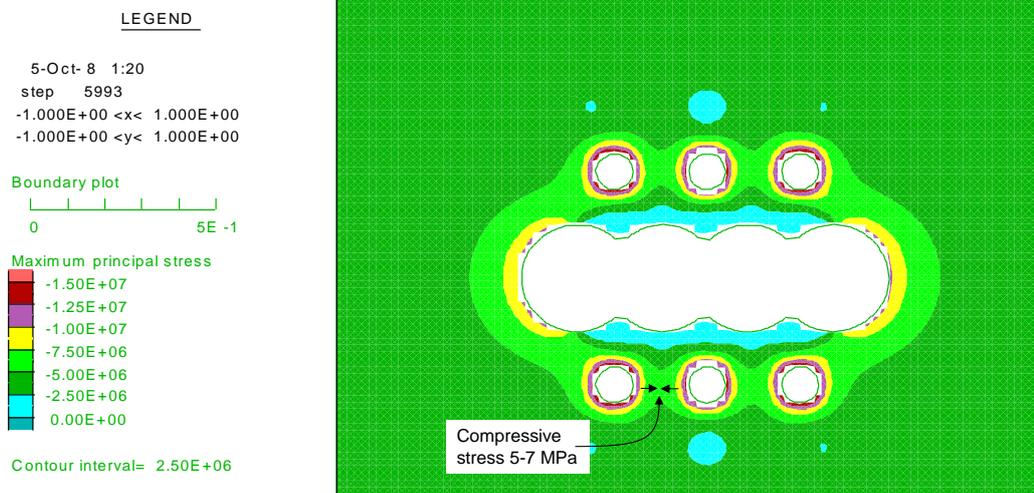
Figure 30: The major principal stress  $\sigma_1$  at 20 MPa pressure in the splitting holes
