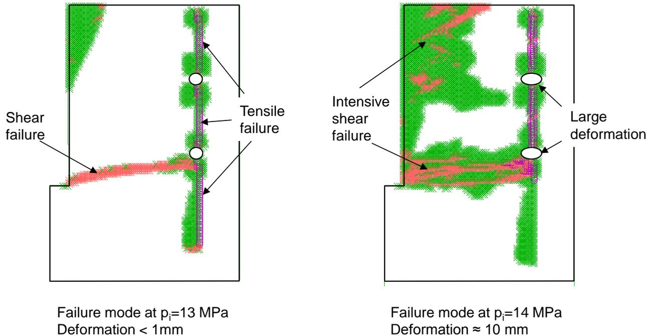
*Figure 24: Simulated failure mode in the numerical model*
