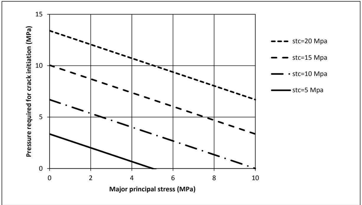
Figure 12: Relationship between rock tensile strength ( $stc$ ), major principal stress  $\sigma_1$  and splitting pressure  $p_s^c$  required for crack initiation (assuming  $\sigma_3 = 0$ )
