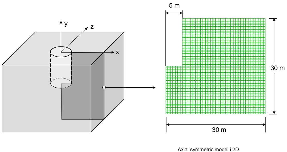
Figure 25: Numerical model for stress analyses around a tunnel face
