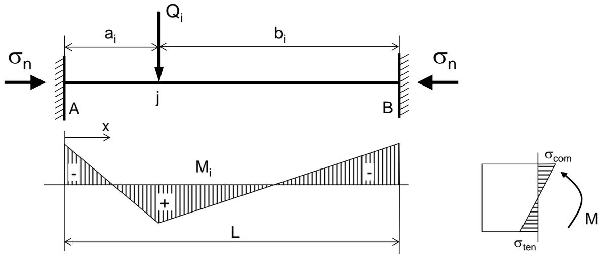
Figure 20: Bending moments caused by one particular load
